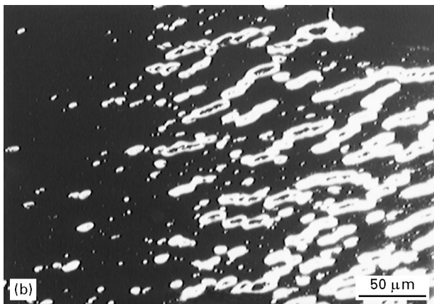
Figure 4 (a) ESEM micrograph of a deformed film at an extension of 7 mm. The population and size of streaks has increased further and the streaks become brighter. (b) ESEM micrograph of a deformed film at an extension of 7 mm, showing a region in which significant cracking has now occurred.
