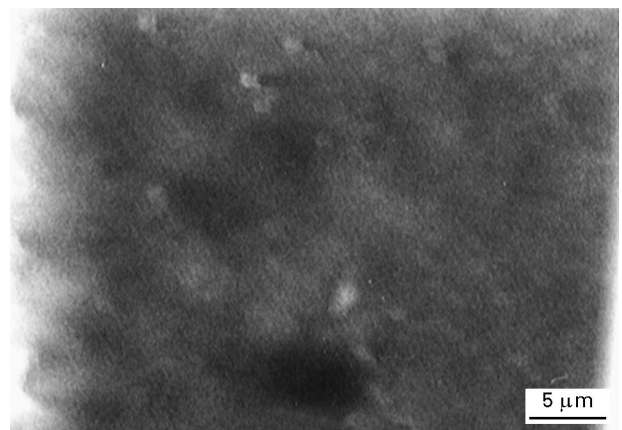
Figure 1 ESEM micrograph of undeformed polymer film, showing a featureless morphology.
